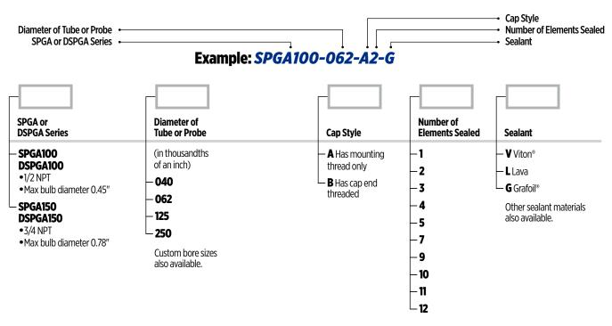
Catalog Numbering System for SPGA and DSPGA
